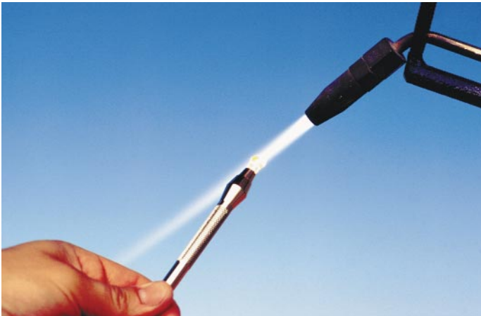
Figure 22. Heating of the glass abutment until it be red and its outlines begin to deform.
