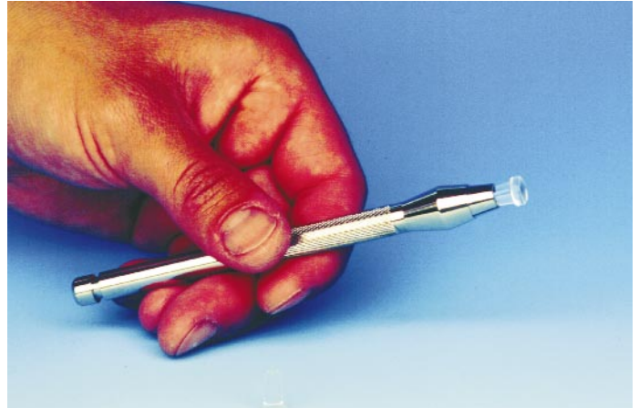
Figure 21. Selection of status corresponding glass sizes and insertion into the clamping apparatus.
